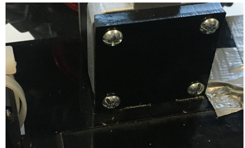
Figure 5: Panels to mount stepper motors to body
